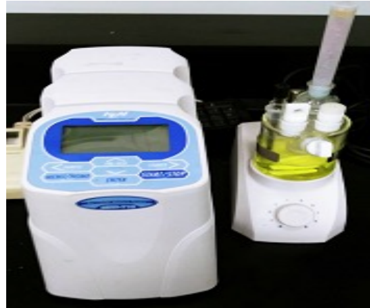
Karl Fischer titrator - Coulomb type - Measuring water content
